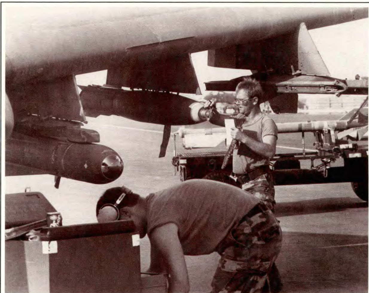
Live combat turn sorties provide realistic training and help maintain the proficiency of both maintainers and flightcrews. Above, a munitions loading team chief checks the arming wire and fuze setting on a 500-pound bomb.
