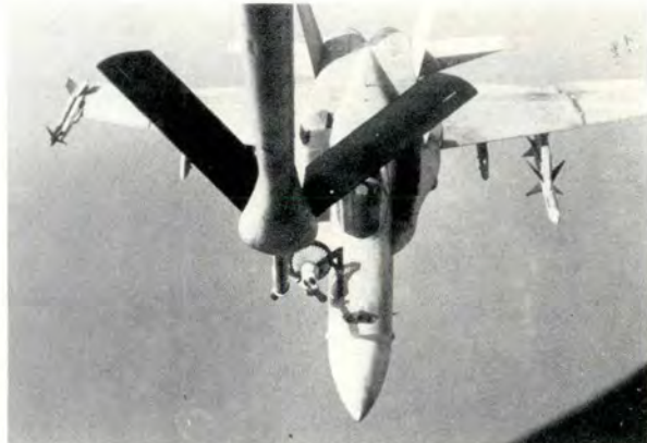
A Marine Corps F-18 receives fuel from an Air Force KC-135 using a probe and drogue.
