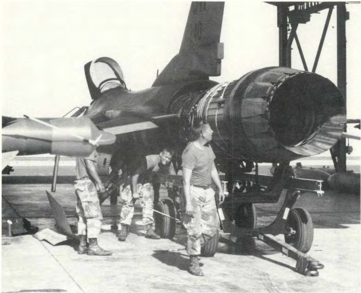
A specialist makes a last-minute check of an F-16 engine before it's installed in the jet following a routine time change.
