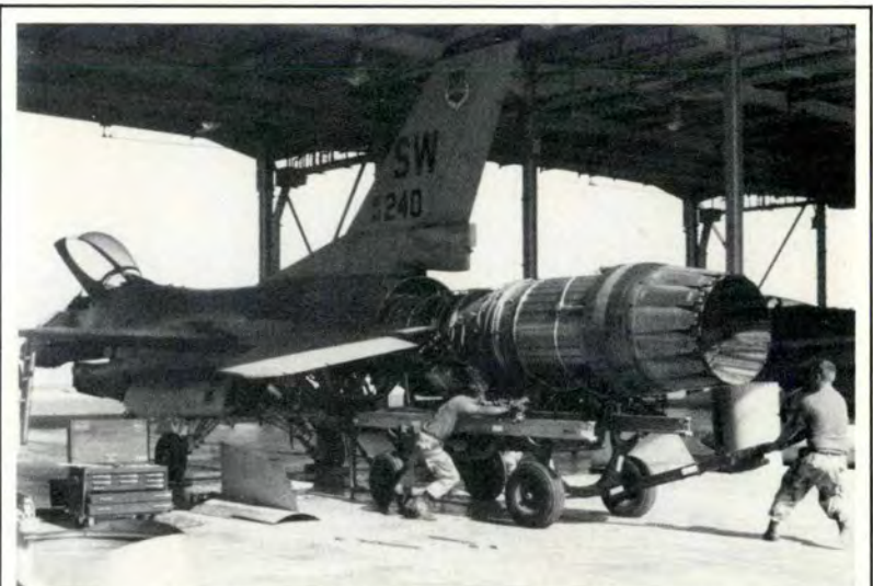
Once removed from the aircraft, the engine will either be repaired on station or shipped for depot maintenance just as it would at home station.
