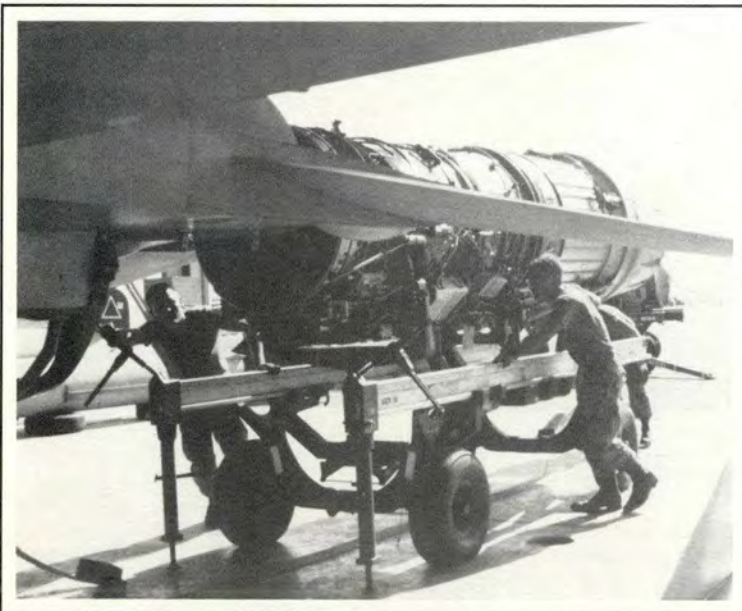
The shade provided by a "T" hangar in the desert makes a routine engine change possible any time of the year. All in a day's work, the aircraft is returned to combat ready status with a new engine.
