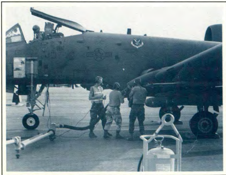
Clear communications and strict adherence to TOs have made for a mishap-free "hot pit" refueling operation.
