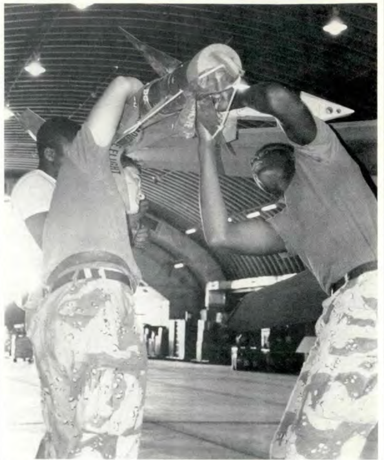
Putting the claws on a Falcon, a munitions load team from the 363 TFW hangs an AIM-9 sidewinder on the wing of an F-16. Over the years, the AIM-9 has proven itself in combat.
