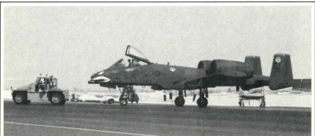
An A-10 is towed from its parking spot to the wash rack. In the desert climate, frequent washings have ensured dust and sand don't keep the aircraft from supporting Operation Desert Shield.
