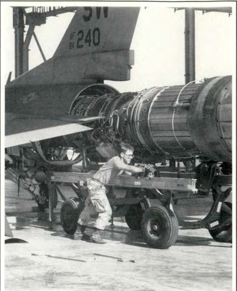
When an engine is due a time change, even in the desert, the specialists can do the job as easily as in the states.
