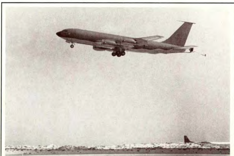
The KC-135R is the newest version of the Air Force's time-proven air refueling jet. CFM-56 engines provide a significant increase in thrust and refueling capability.
